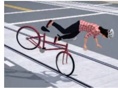
Figure 1 – cycle wheel stuck in rail
